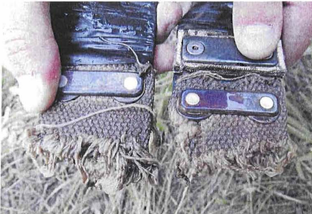
Photo 1: GB726 cotton spacer cut or torn through three punched holes?
