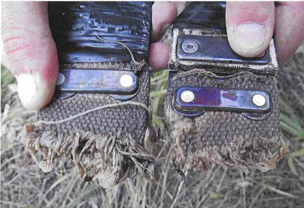
Photo 1: GB726 cotton spacer cut or torn through three punched holes? Note smaller tear near the grommet right of center.
