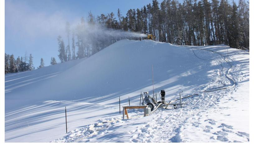
The Gallatin River Task Force manufactures snow as part of a 2011 pilot study that explored snowmaking as an option for disposing of treated wastewater.
